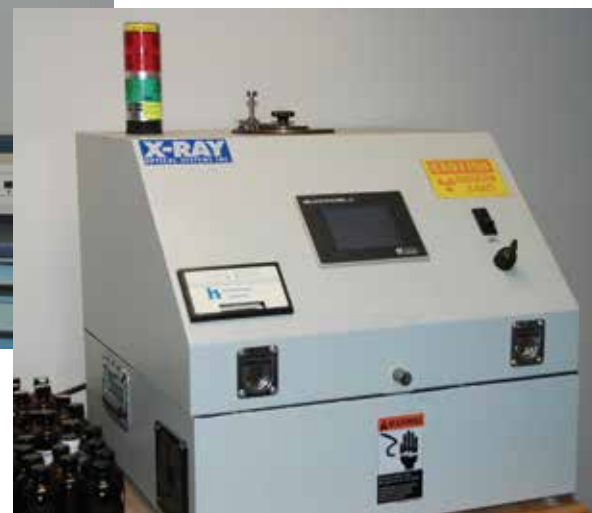
XOS Optical Systems, Sulfur Analyzer (Monochromatic Wavelength-Dispersive X-Ray Fluorescence Spectrometer)
