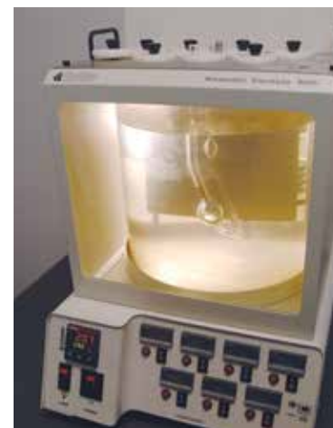
On site Viscosity testing
